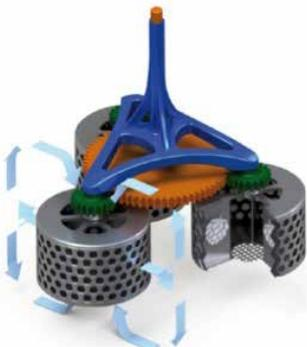
and thereby a directional change of the acting accelerations. The PRBR promises to be a fast, hop-saving and fully scalable technology for dry hopping and other heterogeneous reactions, since it combines efficient mass transfer and filtration in one device. This model sounds very
